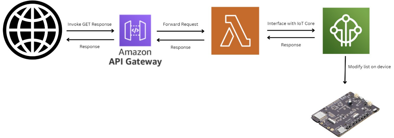
Fig. 2. Cloud component of the PartyBot system. The PartyBot device sends game statistic information to the cloud backend (AWS Lambda) via MQTT communication with AWS IoTCore. The React user interface is connected bidirectionally with the backend via the AWS API Gateway WebSocket API. This architecture facilitates seamless communication between users and the device via the UI, as well as the usage of cloud computing to remove the burden of data processing and game logic from the edge device.
